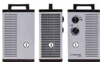
Two air inlets at the front (1) and rear (2) of the heating device supply the powerful radial fan with a high volume of intake air that is then released to the room as warm air current blown through the lateral discharge grille (3).
